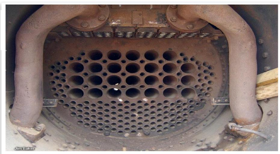
Don't forget the superheater header & main steam pipe NDT examinations
