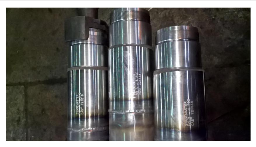
Don't forget the flue tube bottle neck weld(s) NDT examinations
